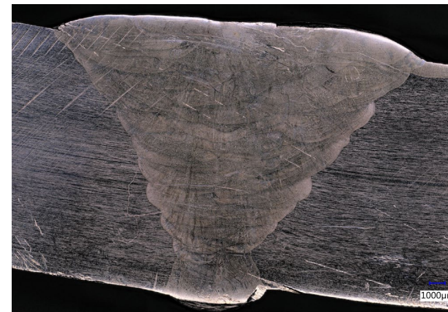
W2: Root: GTAW Cover: GTAW KJ -452°F : 154.2ksiVin
