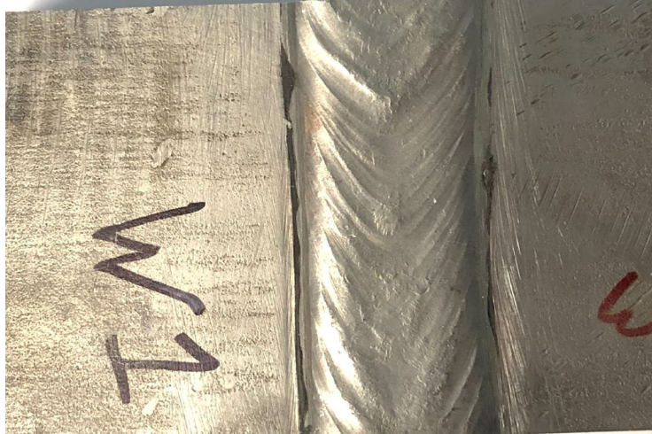
W1: Root: GTAW Cover: FCAW KJ_{-452^{\circ}F} : 58.4ksi/in
