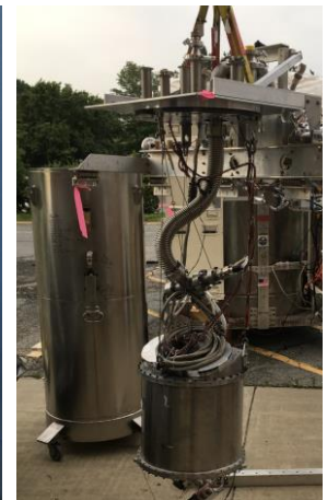
BB integrated into DR system, readout rack and flight-like test facility (PIPER test)
