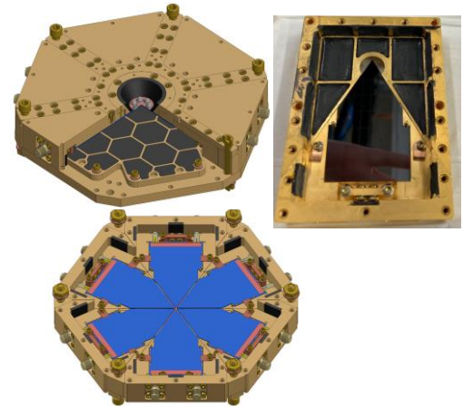
single spectrometer test package and mechanical test chip
