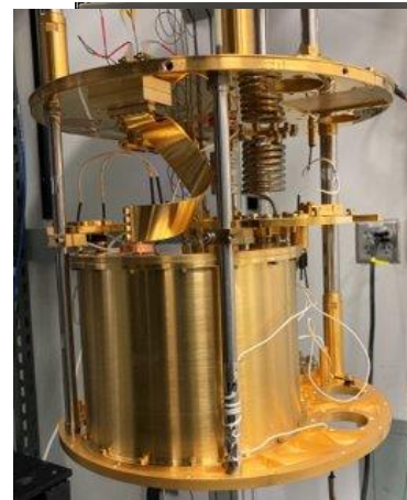
BB integrated into DR system, readout rack and flight-like test facility (PIPER test)
