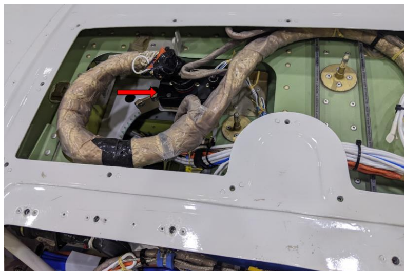
Fig. 3 The MoTeC Synchronous Versatile Input Module (MoTeC USA, Mooresville, North Carolina) in a nacelle of the X-57 airplane.
