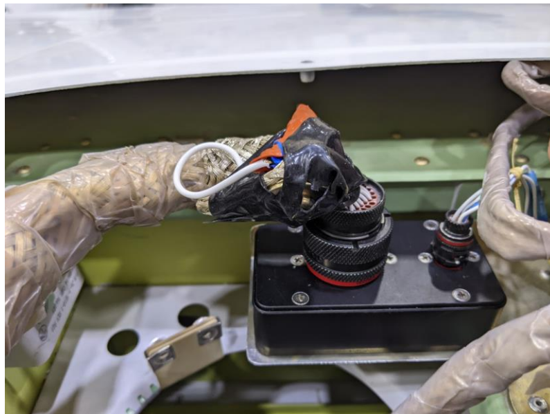
Fig. 5 The X-57 airplane harnessing on the MoTeC Synchronous Versatile Input Module (MoTeC USA, Mooresville, North Carolina).
