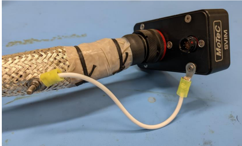
Fig. 4 The laboratory harnessing on the MoTeC Synchronous Versatile Input Module (MoTeC USA, Mooresville, North Carolina).
