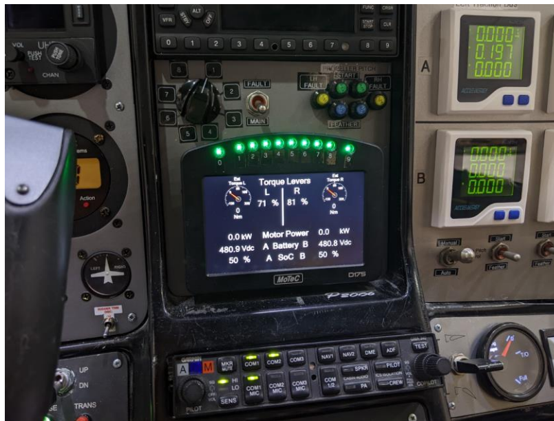
Fig. 1 The MoTeC D175 display (MoTeC USA, Mooresville, North Carolina) in the X-57 cockpit.
