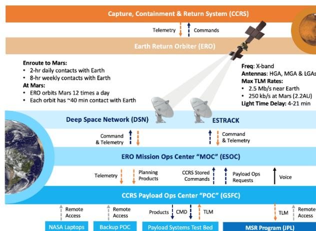
Fig. 6. CCRS ground system architecture.
