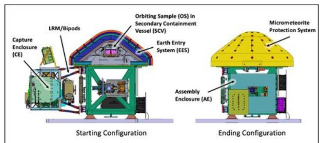
Figure 18. PJR jettison starting and ending CCRS configurations.
