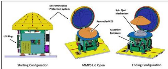
Figure 19. PJR EES release starting and ending CCRS configurations.
