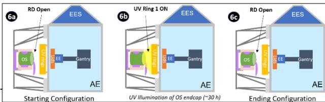
Figure 13. C&C OS base sterilization subphase.
