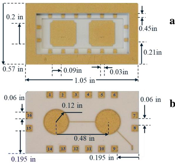
**Figure 1:** Top and bottom views of CF516 package. 1a shows the top side of the package without a lid, 1b shows the package backside. The package is 0.084 in thick.
