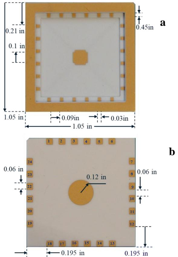
**Figure 2:** Top and bottom views of CF524 package. 2a shows the top side of the package without a lid, 2b shows the package backside. The package is 0.084 in thick.
