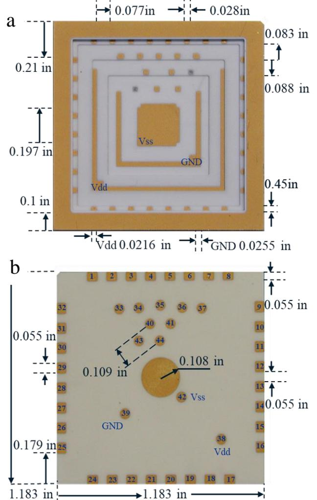
**Figure 3:** Top and bottom views of CF544 package. 3a shows the top side of the package without a lid, 3b shows the package backside. The package is 0.084 in thick.
