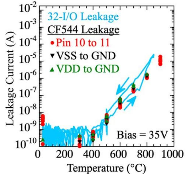
**Figure 4:** CF544 package DC leakage currents compared with previously reported 32-I/O package. Leakage currents through CF544 power bus traces are not significantly any more than other isolated I/Os as the data effectively all plot on top of each other.
