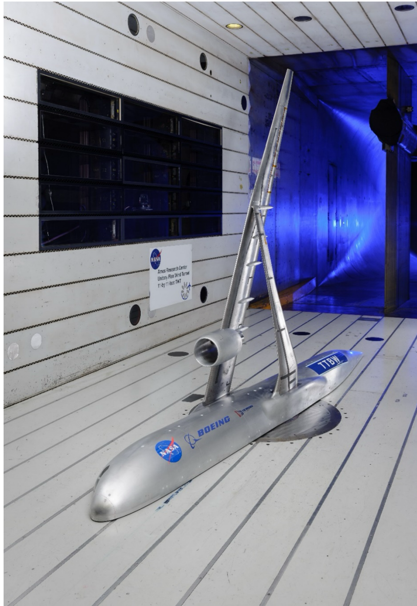
Figure 2-3. 9% Scale Semispan TTBW Wind Tunnel Model installed in the 11-ft Transonic Test Section of the NASA ARC Unitary Plan Wind Tunnel (UPWT) Complex.
