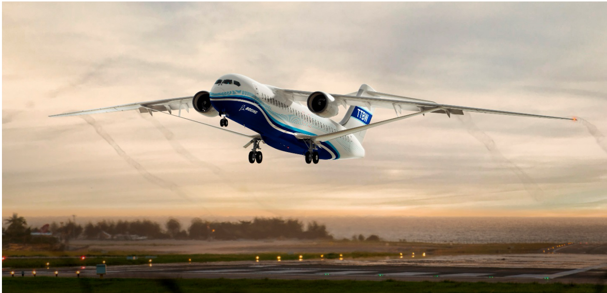
Figure 1-1. The Transonic Truss-Braced Wing (TTBW) Configuration.
