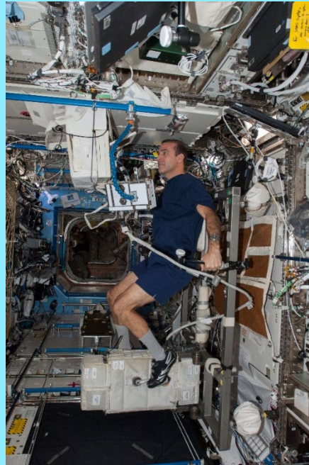
CEVIS (Cycle Ergometer with Vibration Isolation & Stabilization)
