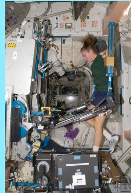
ARED (Advanced Resistive Exercise Device)
