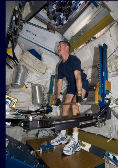
ISS Advanced Resistive Exercise Device- ARED
