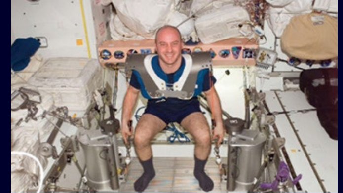
ISS Interim Resistive Exercise Device iRED
