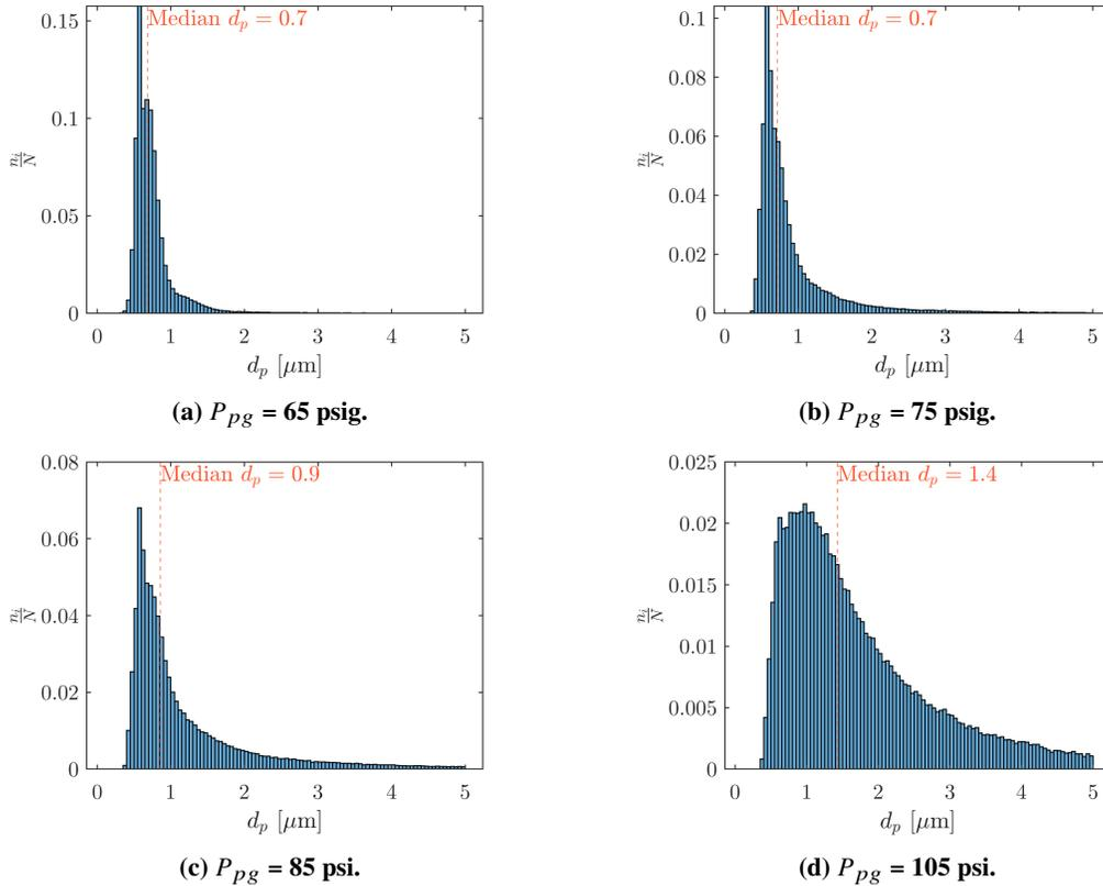
**Fig. 10** Computed particle diameter histograms at  $M_0 = 2.5$  and  $P_{tp} = 70$  psig using PIV vectors computed with  $16 \times 16$  windows at 87.5% overlap.
