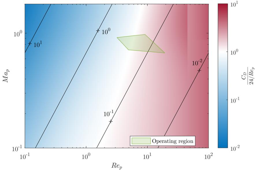
**Fig. 9 Variation in particle drag relative to Stokes' model[15] showing operating boundaries of the current test.** Lines of constant  $Kn$  are shown in black and labeled. Test conditions from Table 1 and a particle size range of  $0.3\text{--}1.0 \mu\text{m}$  were used to generate operating region bounds.
