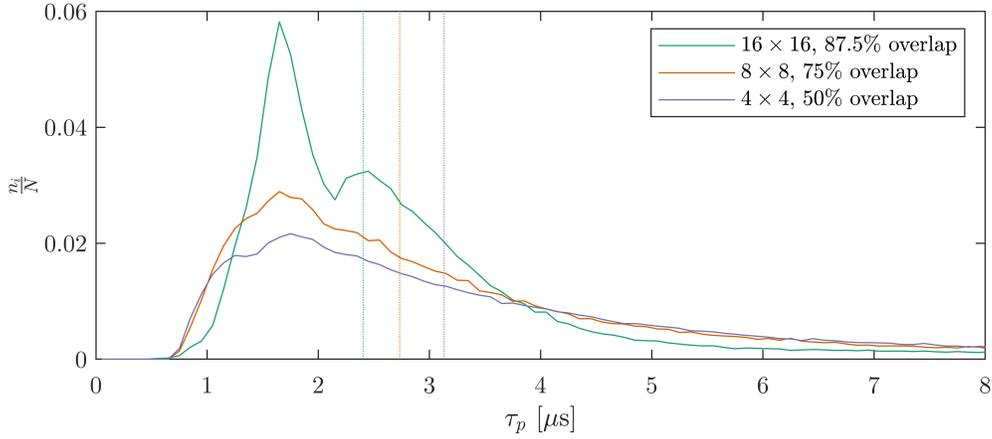
**Fig. 8 Particle relaxation time probability density distributions with varying PIV interrogation window parameters.** Same dataset as Figure 7. Dashed lines show median value for each distribution.
