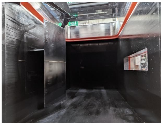
**Fig. 2 18° wedge model installed in the 1'x1' Wind Tunnel test section (forward looking aft).**
