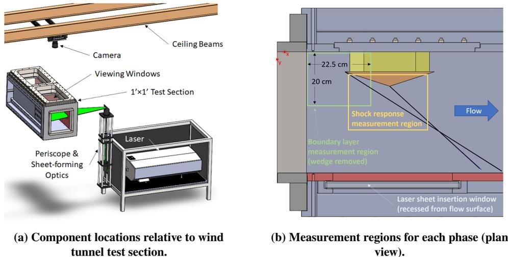
**Fig. 6 PIV system arrangement.**
