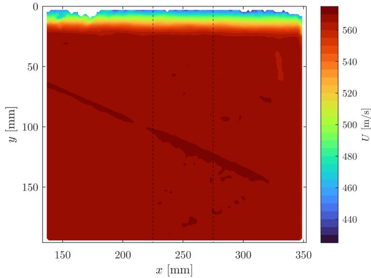
**Fig. 13 Sidewall boundary layer mean flowfield at  $M_0 = 2.5$  maximum Reynolds number condition.**
