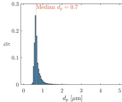
**Fig. 11** Computed particle diameter histogram at optimal operating condition ( $P_{pg} = 65$  psig,  $P_{tp} = 70$  psig) for  $M_0 = 3.5$  using PIV vectors computed with  $16 \times 16$  windows at 87.5% overlap.
