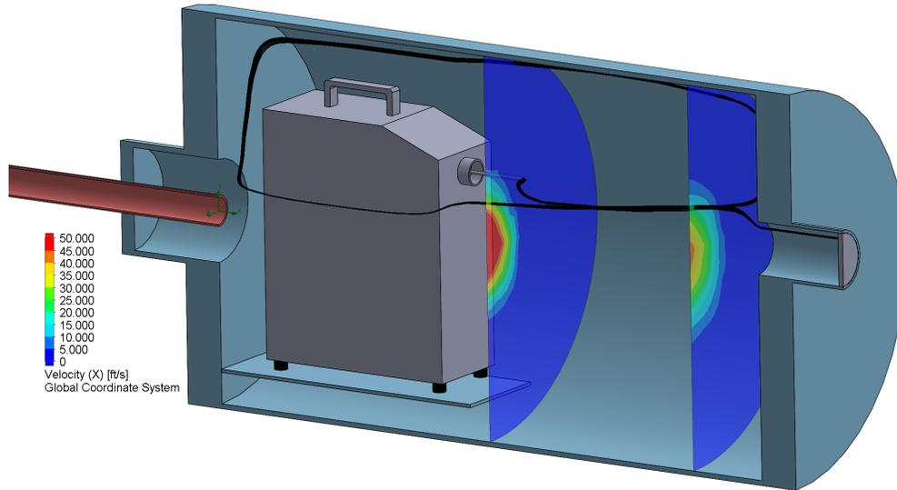
**Fig. 4** CFD solution for legacy PIV particle seeding tank configuration with increased purge air capability. Particle generator arrangement and tank are symmetric about the section plane.
