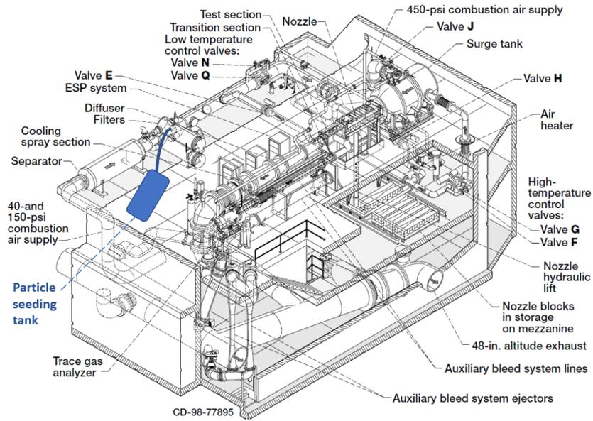
**Fig. 1 Diagram of the 1'x1' Supersonic Wind Tunnel facility highlighting the location of the particle seeding tank in the basement[8].**
