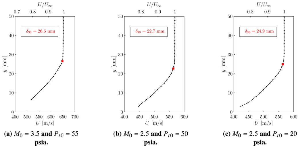
**Fig. 14 Sidewall boundary layer velocity profiles at  $x = 25$  cm.**
