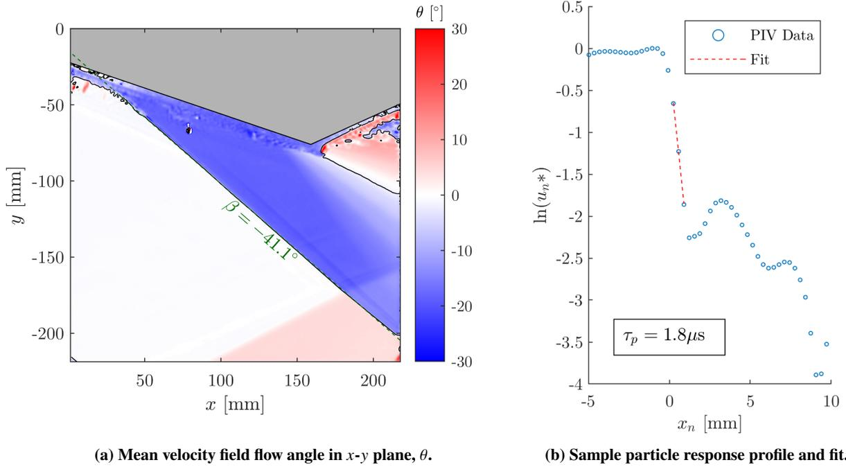
**Fig. 7 Shock response velocity field at  $M_0 = 2.5$  and  $P_{pg} = 65$  psig using  $16 \times 16$  windows and 87.5% overlap.**
