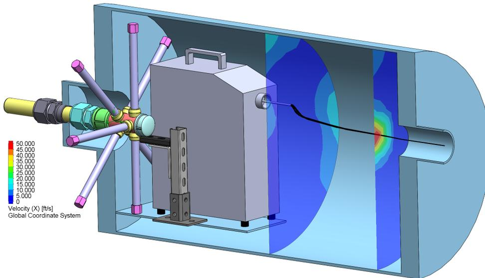
**Fig. 5** Upgraded PIV particle seeding tank configuration operating at 2 lbf/s of buffer flow. Particle generator arrangement and tank are symmetric about the section plane.
