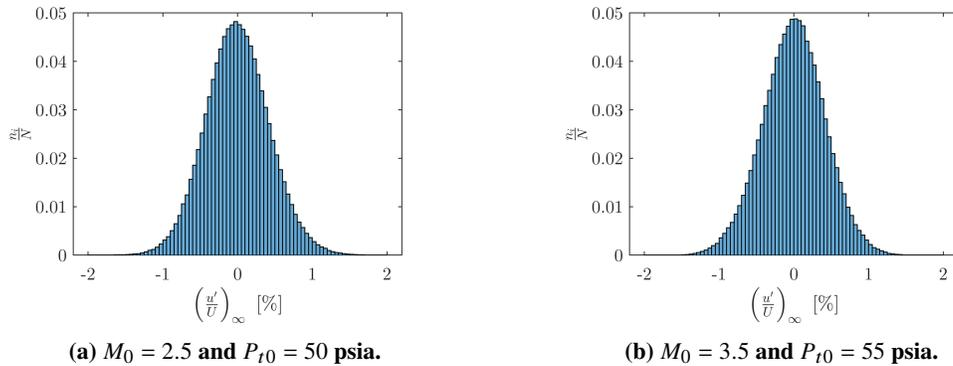
**Fig. 16 Freestream ( $y > 2\delta_{99}$ ) velocity fluctuation distributions.**
