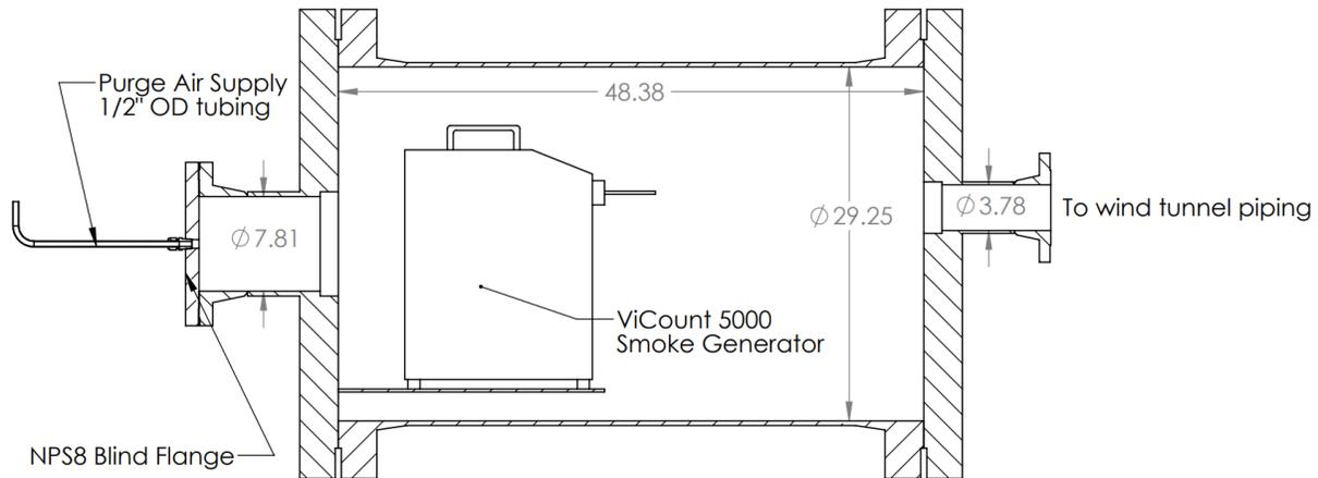
**Fig. 3 Elevation section view of legacy PIV particle seeding tank configuration.** *Particle generator arrangement and tank are symmetric about the section plane.*
