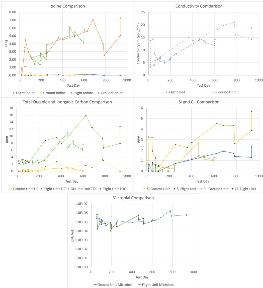
**Figure 2. Various final water quality results of the SERFE Flight and Ground Units.**
