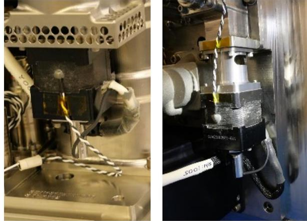
**Figure 8. Body rust on linear actuators of SWME BPV (left) and TCV-421 (right).**
