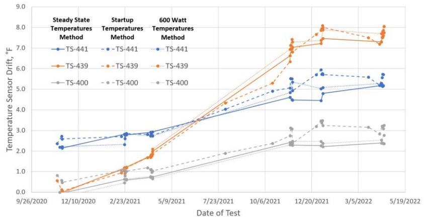
**Figure 11. Estimated temperature sensor drift of three major sensors on the SERFE Flight Unit.**
