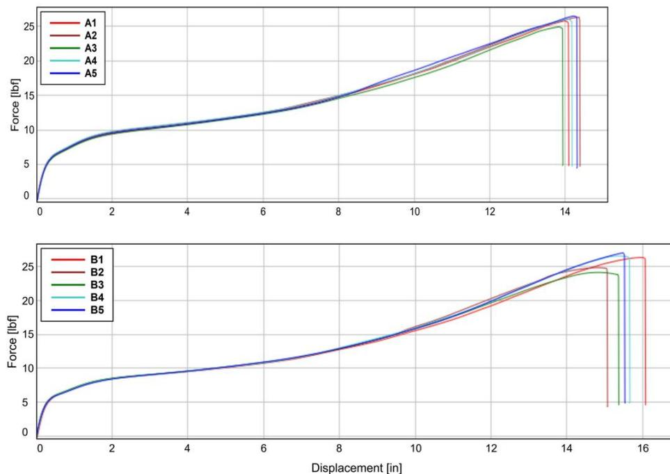
**Figure 12. LCVG tubing mechanical testing results for a non-specific, untreated sample set (top) and a sample set from the SERFE Flight Unit following disassembly.**
