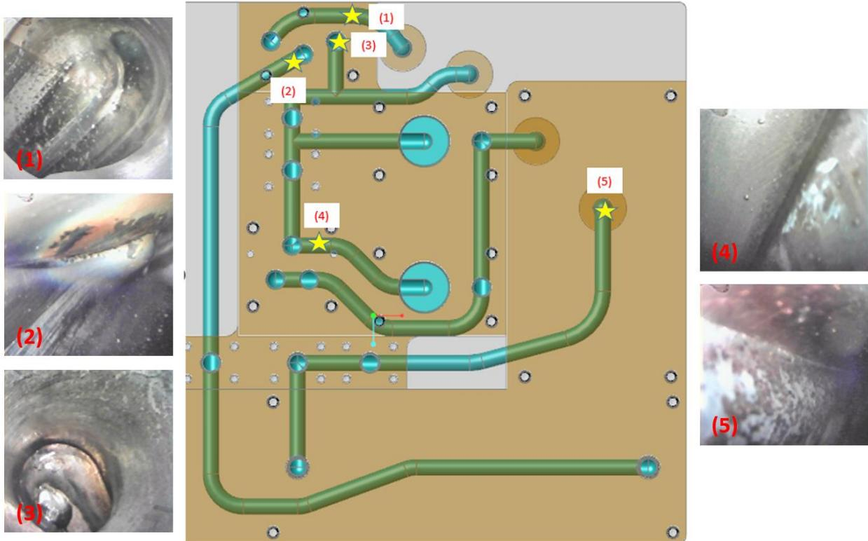
**Figure 10. Areas of interest on backplate including the TCV LCG outlet (1), TCV inlet (2), TCV pump outlet (3), PMP-422 inlet (4), and HX-440 inlet (5).**
