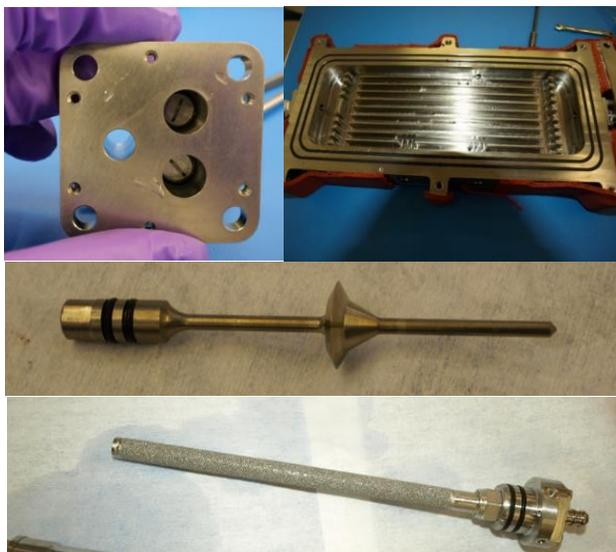
**Figure 7. Various SERFE components following removal, including RV-424A/B (top-left), heater assembly (top-right), TCV-421 shuttle (middle), and F-2048 (bottom).**
