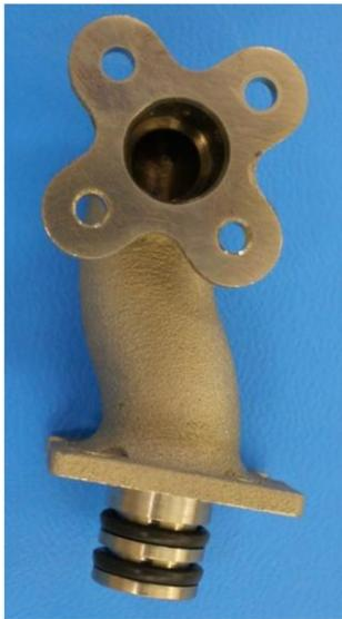
**Figure 9. Presumed rust spots on secondary pump manifold.**
