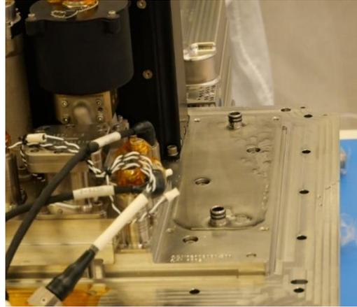
**Figure 4. Water puddle beneath HX-440.**
