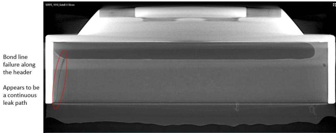
**Figure 6. SWME Cartridge Bond Line Failure**
