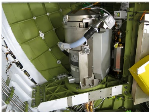
Fig. 1. Orion UWMS installed in Artemis-II Vehicle
