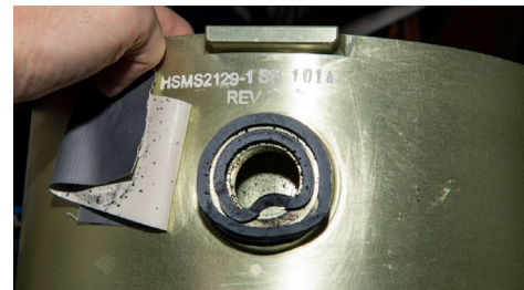
Figure 6. Toilet Air Filter inlet seals after improper installation.
