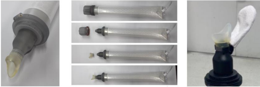
Figure 13. Evaluation #4 Backup Urine System (BUS) prototypes - female interface (left) female interface installed on BUS with cap on/off (middle), and menses collector (right).
