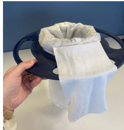
Figure 4. Artemis Bag with “wipe” feature to aid in initial fecal separation. Evaluated during evaluation #4.
