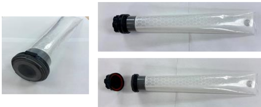
Figure 14. Evaluation #4 Backup Urine System (BUS) prototypes with the male interface (left) and BUS male interface with cap on/off (right).
