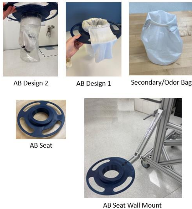
Figure 12. Evaluation #4 Artemis Bag - two prototype designs including hand-held and wall mounted seat.
