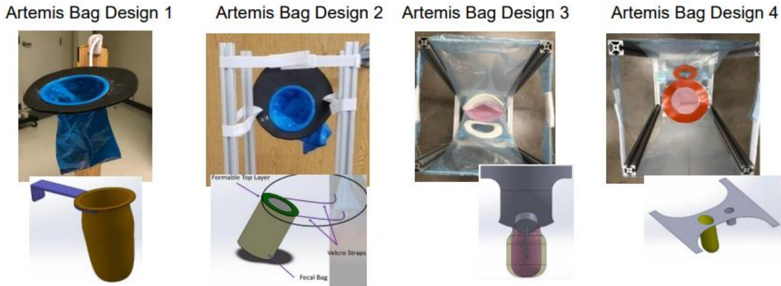
Figure 8. Evaluation #1 Artemis Bag Low-Fidelity prototypes. Four different designs were evaluated.
