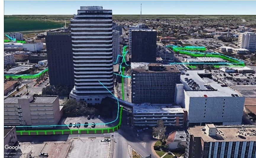
Ground truth (green) and computed position from receiver data (cyan) on June 6.
