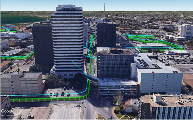
Ground truth (green) and computed position from receiver data (cyan) on June 6
