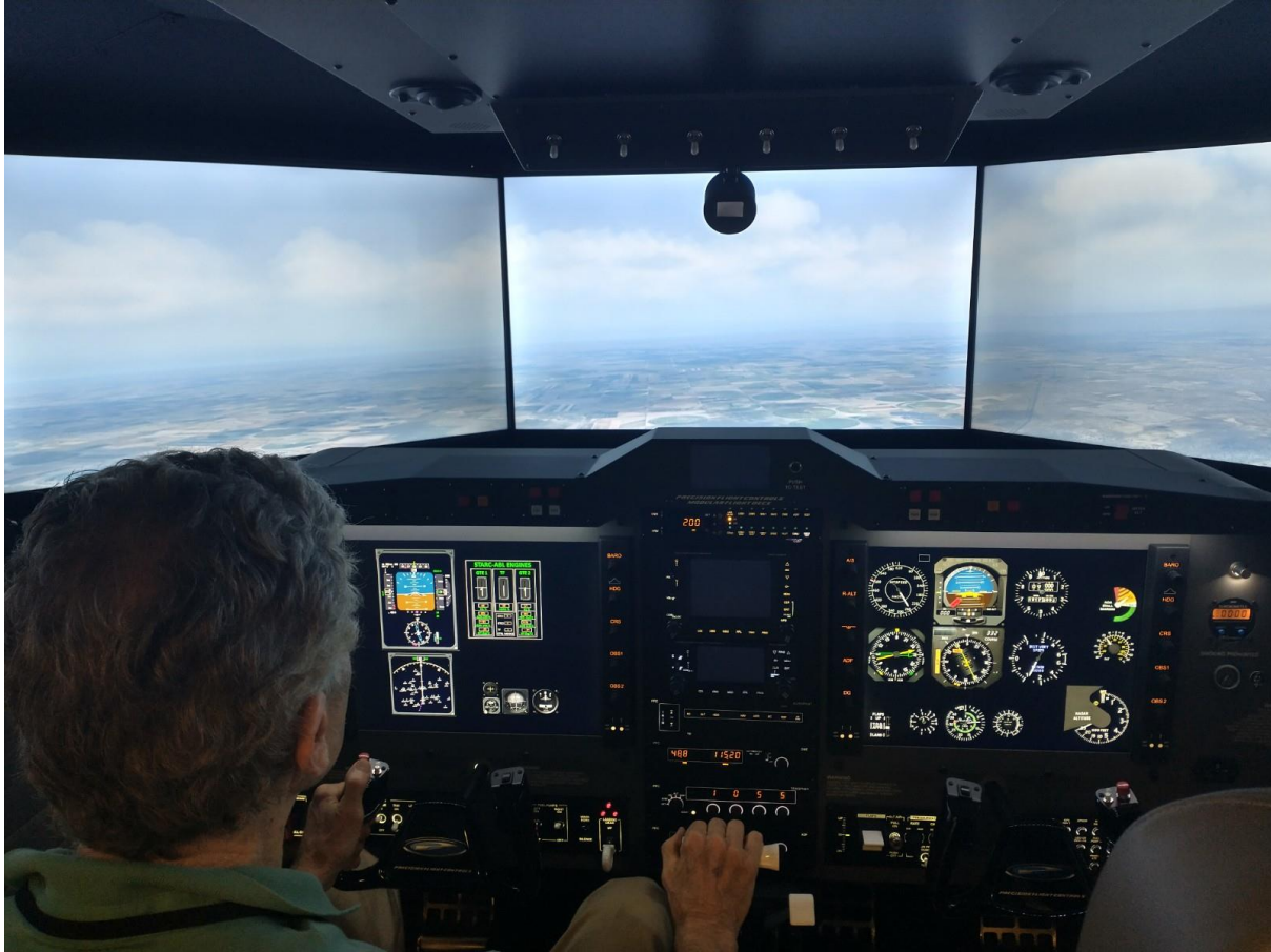
Figure 5. Piloted testing of reversionary control modes in flight simulator.
