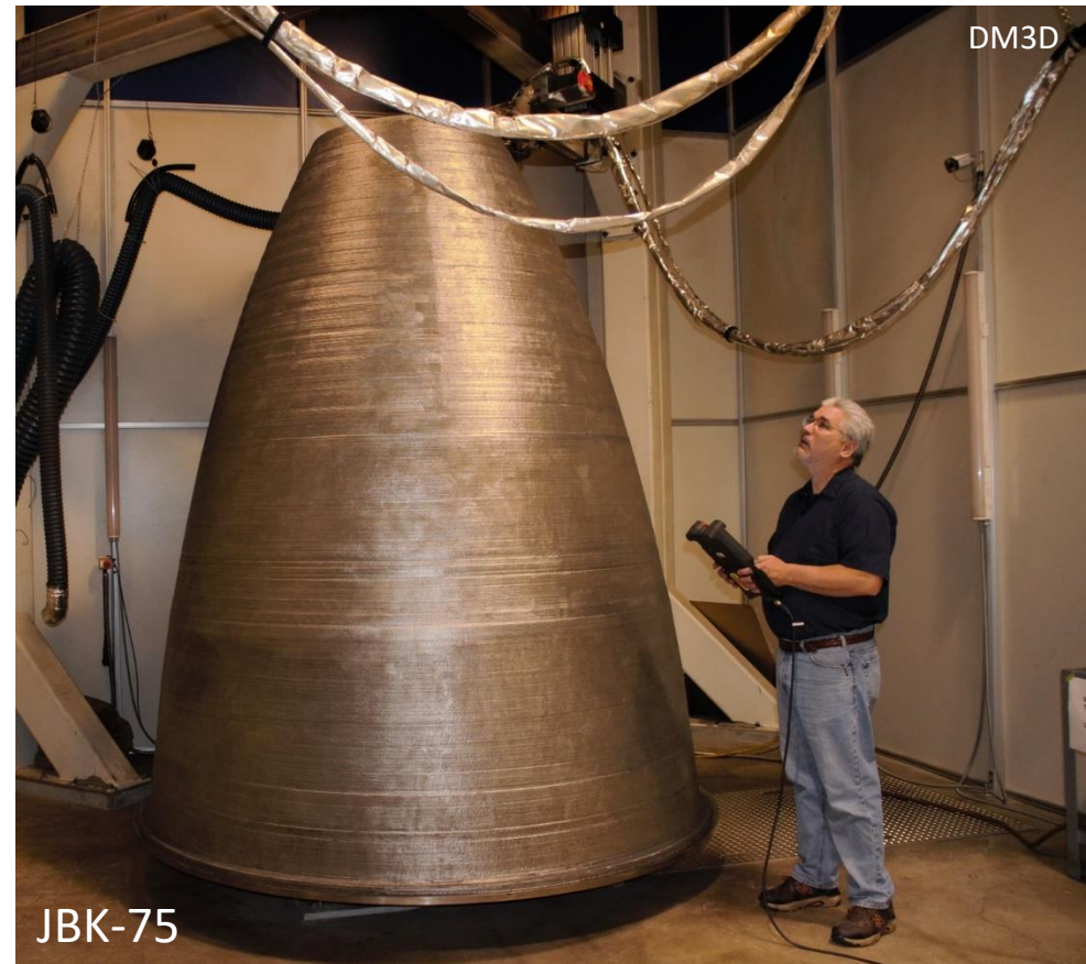
95" (2.41 m) dia and 111" (2.82 m) height Near Net Shape Forging Replacement
