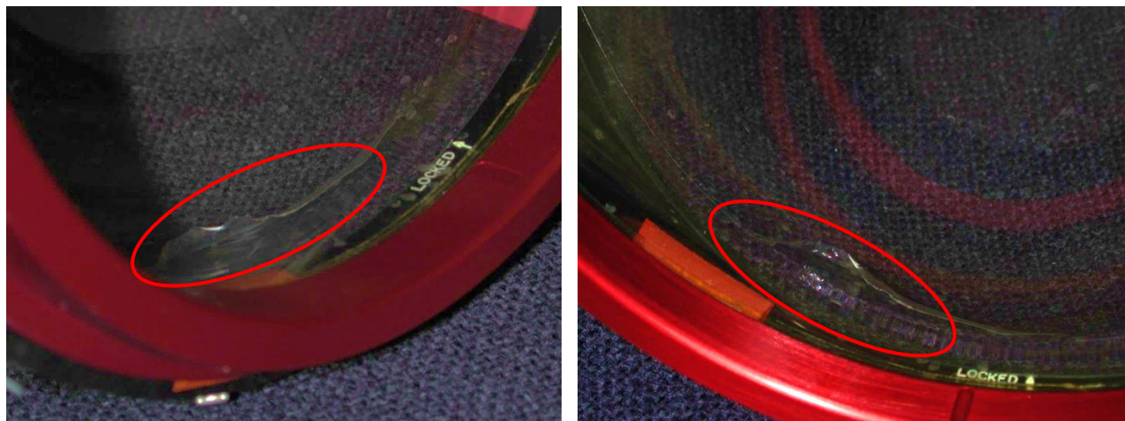
Figure 1: Delamination of the HTAF-308 coating after NBL testing.
