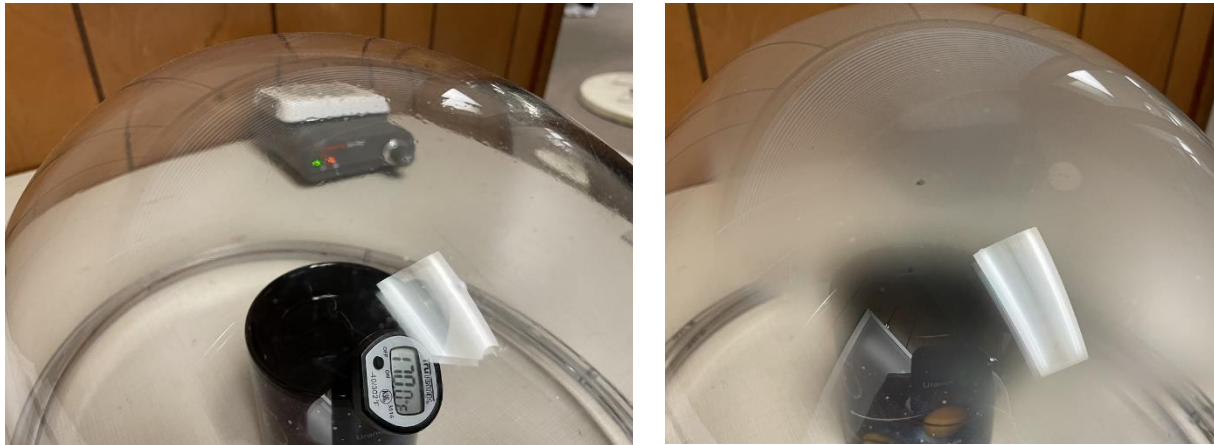
Figure 10: Visgard (Left) versus HCF-100 (Right) when exposed to 170 deg F hot water While the HCF-100 fogs more to the 170 deg F water, the Visgard develops an orange peel texture that starts to streak. This could be a concern for eye irritation.
