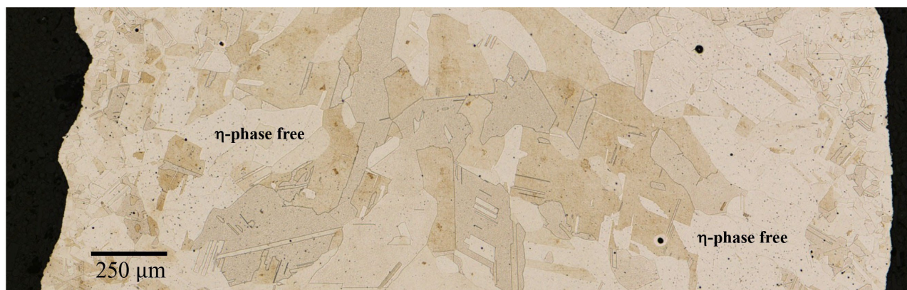
Figure 13. Macrostructure of a 3.175 mm thick single-pass LP-DED NASA HR-1 panel after homogenization at 2175 °F/3h. The as-homogenized sample appears free of \eta -phase.
