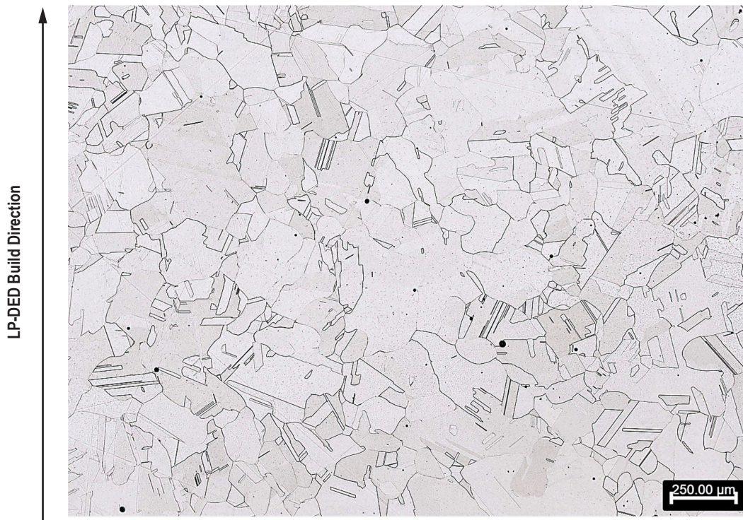
Figure 38. The typical microstructure (in x-z plane) of the LP-DED NASA HR-1 samples used for tensile testing in 5 ksi gaseous hydrogen environment. The average grain size is approximately 75\ \mu\text{m} .
