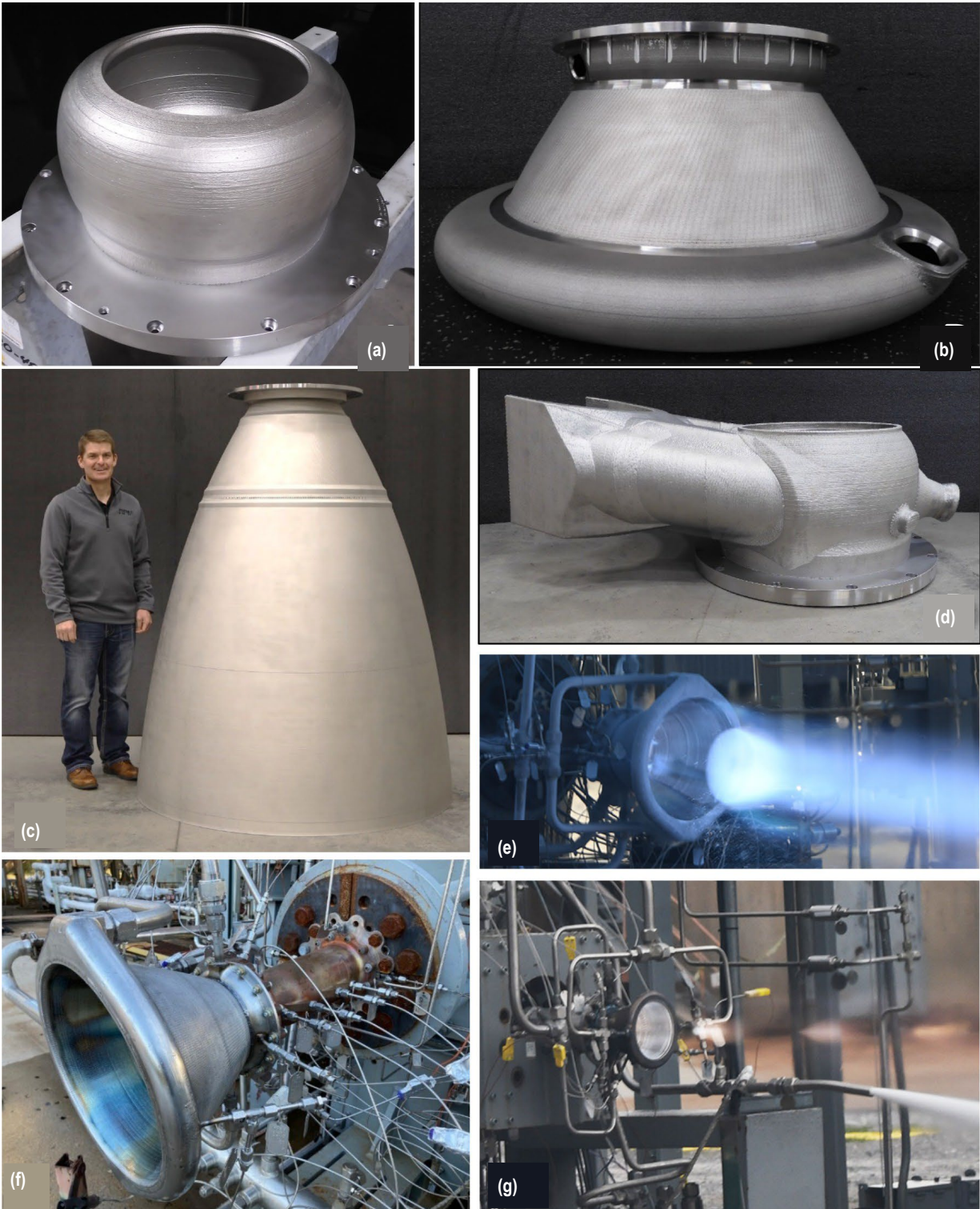
Figure 55. Examples of various NASA HR-1 LP-DED components. (a) Domes for powerhead, (b) 35K-lbf nozzle with integral channels and welded manifolds, (c) Integral channel wall nozzle, (d) Powerhead half shell, (e) Hot-fire testing of regeneratively-cooled nozzle for LLAMA, (f) 7K-lbf nozzle for LLAMA, (g) High duty cycle testing of integral channel nozzle to 207 starts.
