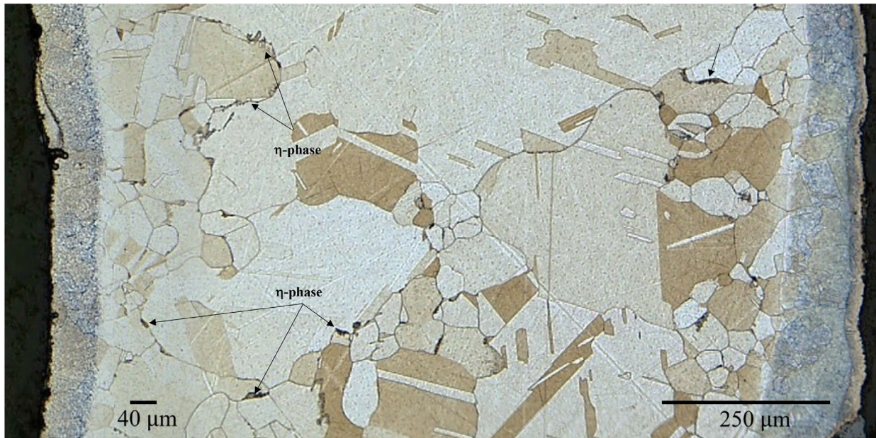
Figure 16. Grain-boundary \eta -phase is more evenly distributed in a thin single-pass LP-DED NASA HR-1 panel (1 mm thick) after being aged at 1325 °F/16h. This 1 mm thick single-pass LP-DED panel was deposited at a laser power of 350 watts.
