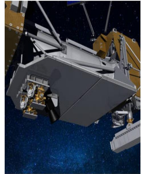
The LCRD payload is attached to the LCRD support assembly flight (LSAF), depicted in this illustration. The LSAF serves as the backbone for LCRD's components. Attached to the LSAF are a star tracker and two optical modules (left), which generate the infrared lasers that transmit data to and from Earth. Other LCRD
