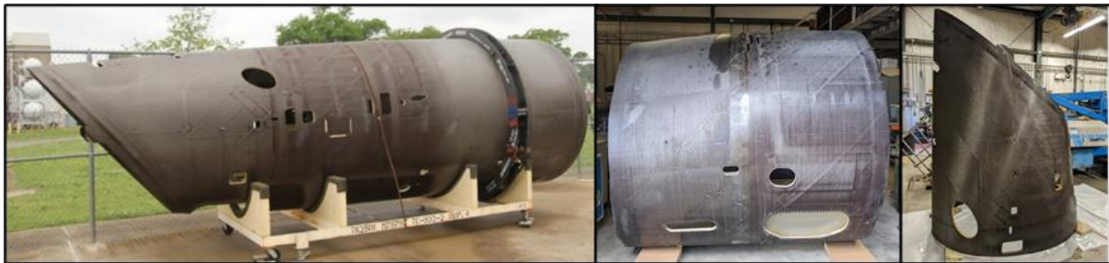
Figure 1. Hawker 4000 fuselage section: original fuselage (left), forward section (middle), and aft section (right)
