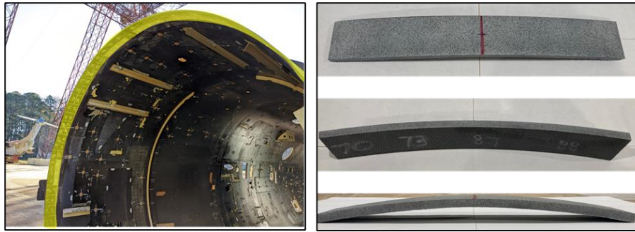
Figure 2. Hawker 4000 forward composite flange (left) and cut test specimens (right).
