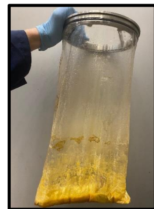
Figure 9. Brine/foam left after 99% water recovery.
