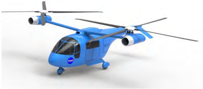
Side-by-Side (Intermeshing Rotors) [1]
