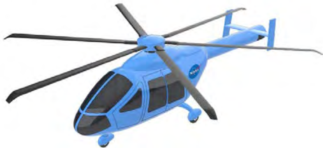
Quiet Single-Main Rotor (QSMR) (NOTAR, specifically designed for quiet operations) [3]
