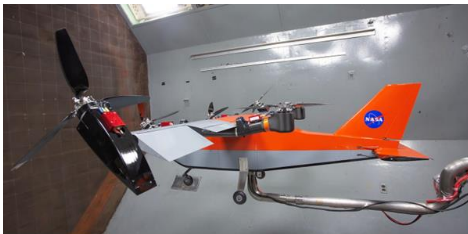
Fig. 9 The SWFT-1 aircraft in the NASA Langley 12-Foot Low-Speed Tunnel, shown here with forward and tip propellers partially tilted and flaperons partially deflected.
