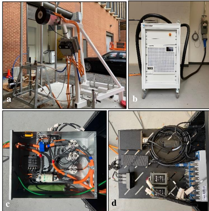
Fig. 7 Powertrain test stand. (a) Fully integrated test stand with motor and inverter, (b) 54 kW DC power supply (c) high-voltage electrical components including contactors, fuses, and current and voltage sensors, (d) data acquisition and control components.
