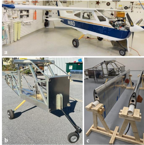
Fig. 3 Bede BD-6 [7]. (a) BD-6 aircraft, (b) Rolling fuselage frame owned by Georgia Tech, (c) Tubular spar and bonded rib wing owned by Georgia Tech.
