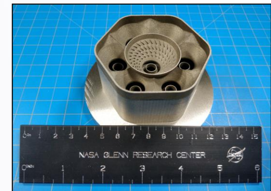
3D-printed ODS Combustor Dome
