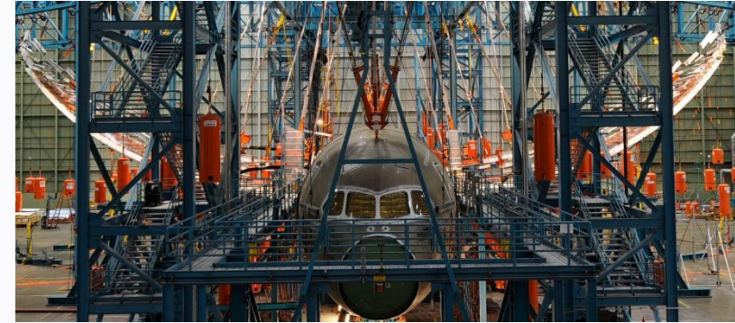
787 Wing Flex During Testing
