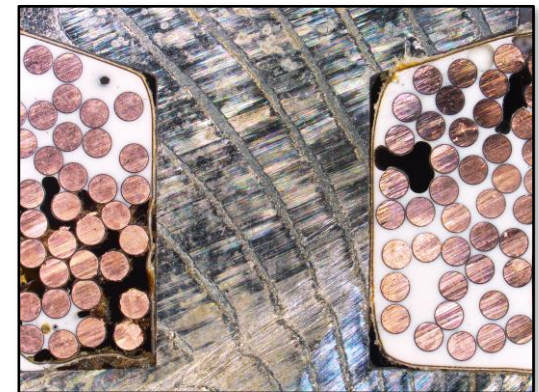
Improved fabrication process still exhibits some voids
