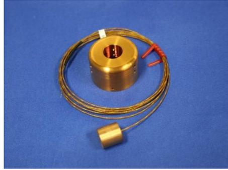
**Fig. 4 Copper slug calorimeter.**
