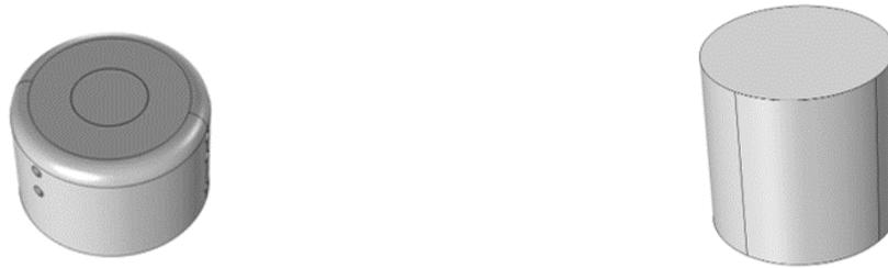
(a) Slug Calorimeter Model (with Housing).
