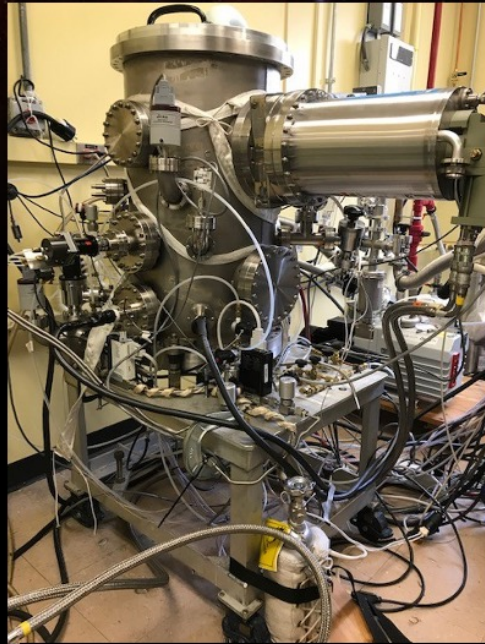
UHV chamber for PVD thin-film deposition with XeF 2 fluorination.
