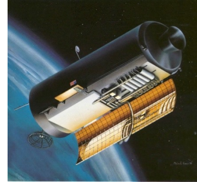
Air Force BSTS DIPS 6 kWe, 675 kg
