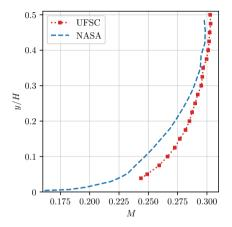
◎ Different flow profiles were observed in each test rig, the boundary layer displacement thickness was evaluated as  $\delta^*_{\text{UFSC}} = 1.02 \text{ mm}$  and  $\delta^*_{\text{GFIT}} = 2.60 \text{ mm}$ .
