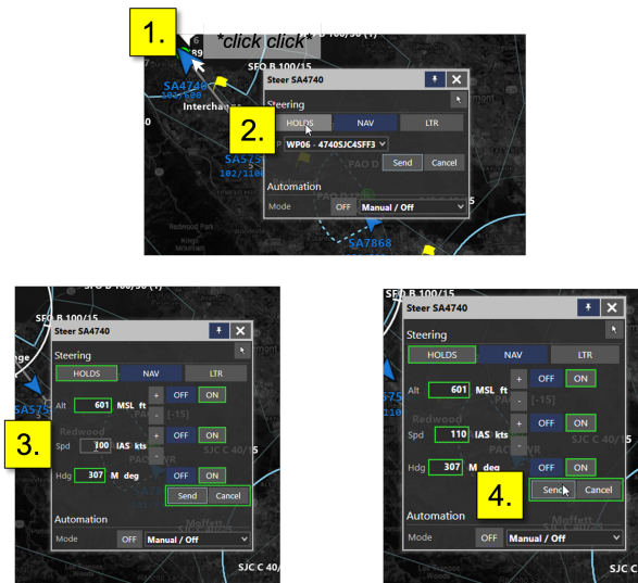
Fig. 6 Sequence of actions required to upload a new maneuver to a vehicle in response to an ATC call in the Voice condition.
