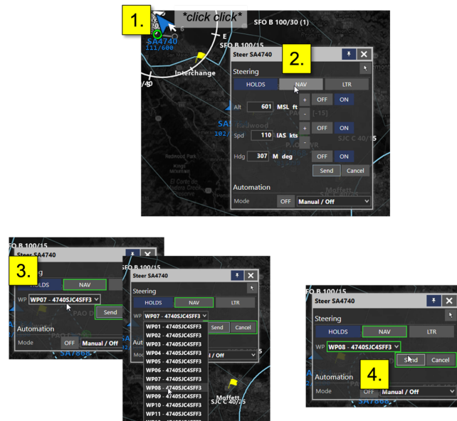
Fig. 6 Sequence of actions required to upload a new maneuver to a vehicle in response to an ATC call in the Voice condition.
