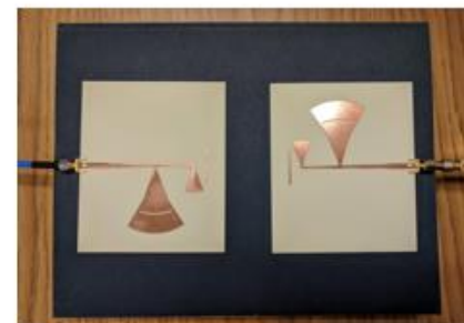
RF Power Harvesting Antennas- UAH
