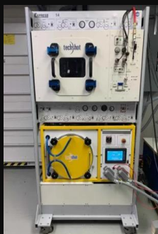
ISS Demo – Fablab Manufactures both Metal and electronic components on orbit
