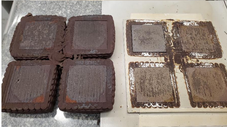
3D printed ablative material does not stick to aluminum or titanium
