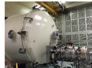
Marshall 100 Meter X-ray Beamline: left: beamline; right: instrument chamber with bell housing
