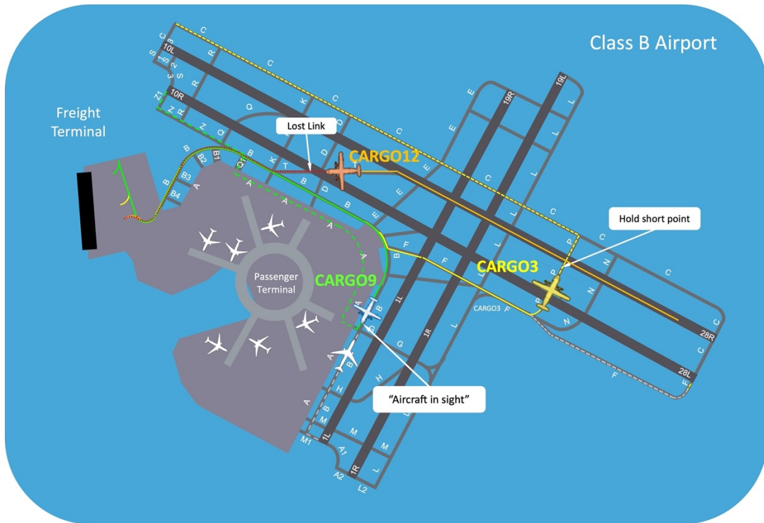
Figure 8. Surface operations overview graphic depicting CARGO3, CARGO9, and CARGO12 at a Class B airport.
