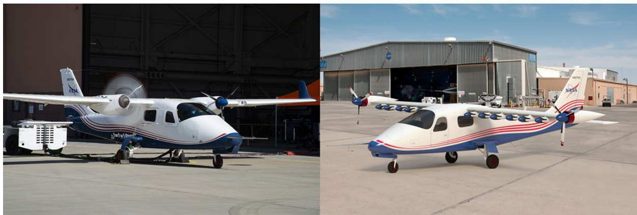
Fig. 2 Picture of the X-57 in the Mod II configuration with cruise propellers mounted on inboard nacelles (left), and a rendering of the X-57 in the Mod III/IV configuration with cruise propellers mounted on wingtip-mounted nacelles (right).
