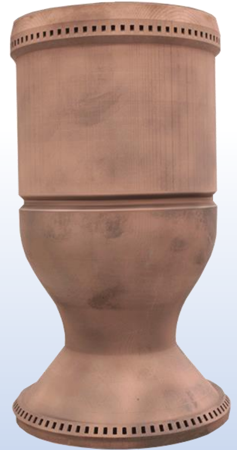
30,000 lb f class GRCop-84 combustion chamber liner made from L-PBF
