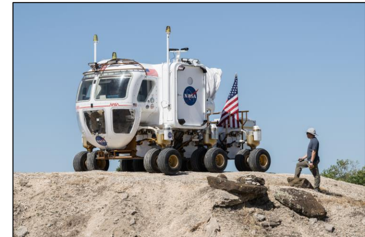
NASA's 6-wheeled pressurized rover (PR) testbed was updated to test drive-by-windows & drive-by-cameras driving modes
