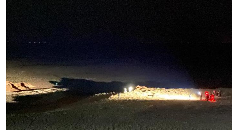
High-Intensity Light Simulated Low-Angle Sun at Lunar Poles
