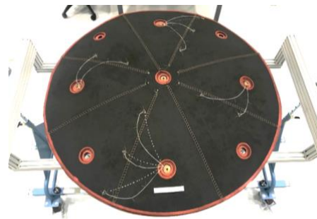
Fig 1. Thermocouples and Heat Flux Gages Integrated with LOFTID Nose Insulation.
