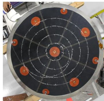
Fig 1. Thermocouples and Heat Flux Gages Integrated with LOFTID Nose Insulation.
