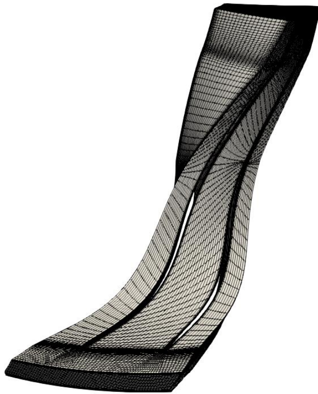
Figure 13: Computational domain for impeller
