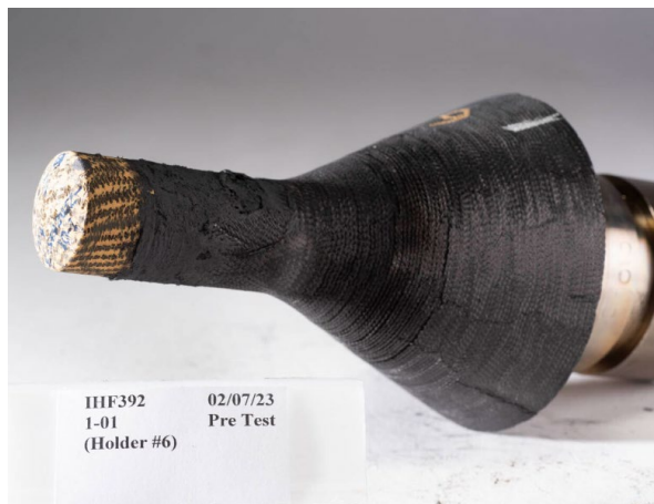
Figure 1. 1-inch diameter iso-q 3MDCP article (striped) assembled in carbon-phenolic holder (black).
