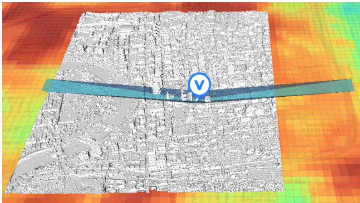
Figure 2† (a): City of Columbus, OH, building heights from LIDAR data, and the approach and departure surfaces.
