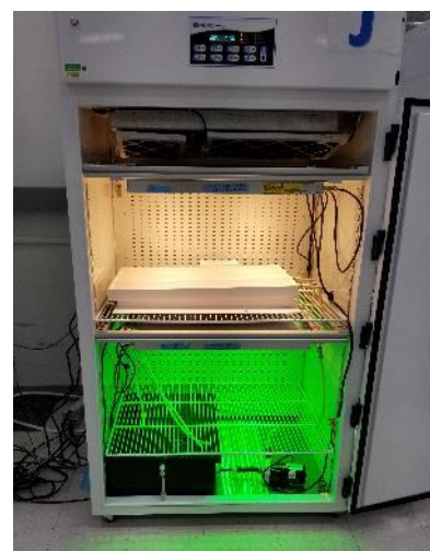
Figure 1. Microgreen cultivation system installed in reach-in controlled environmental growth chamber. Here, lower tray is removed to view nutrient solution tank and pump.
