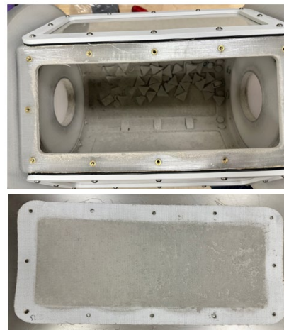
Figure 2. Interior of Rotational Tumbler (top) and Abraded panel of Ortho Fabric (bottom).
