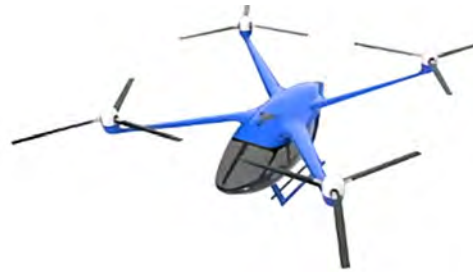
Fig. 2 NASA's quadrotor urban air taxi [3].
