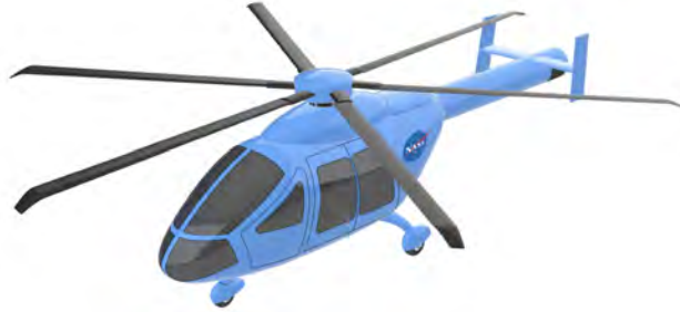
Fig. 1 Rendering of the quiet single-main rotor helicopter design for UAM.
