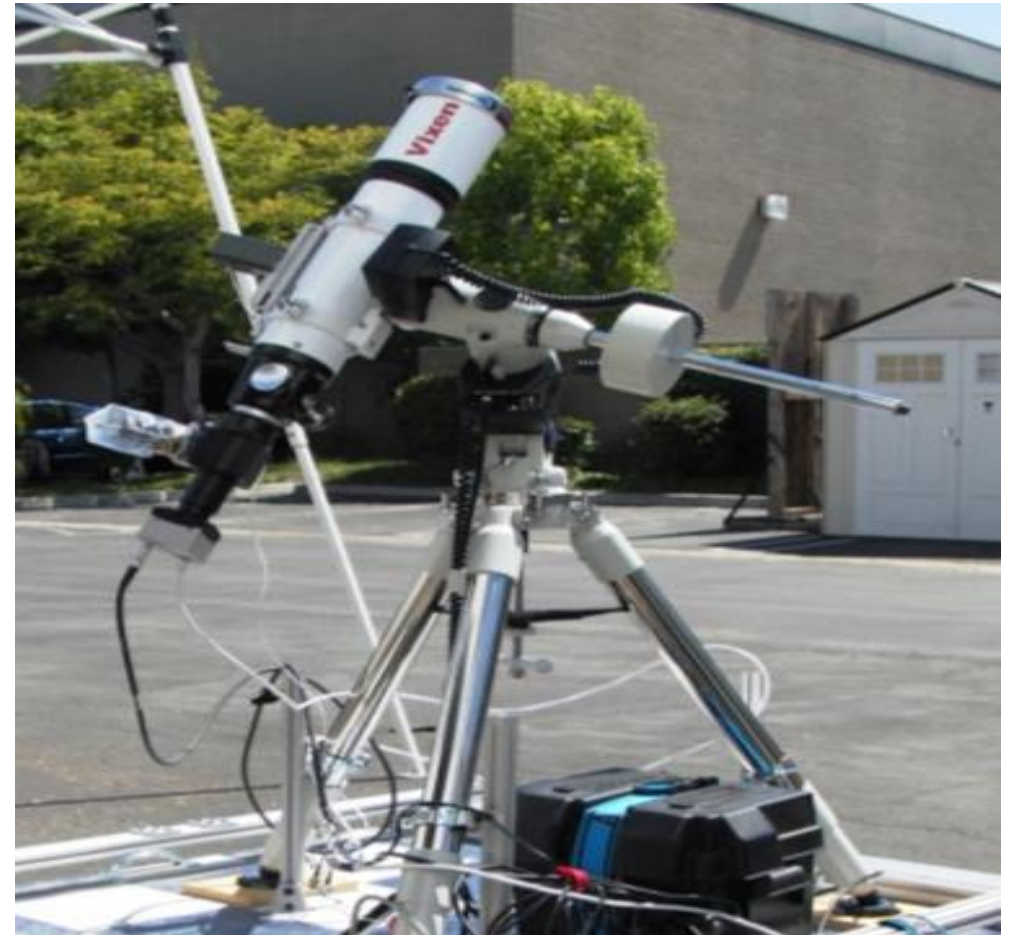
Off-the-shelf telescope with tracker and high-speed camera
