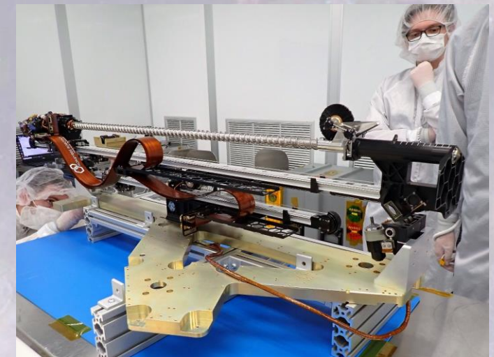
TRIDENT mounted on Intuitive Machines 3PO Pallet
