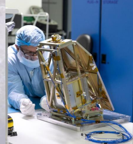
MSolo on vibration test fixture
