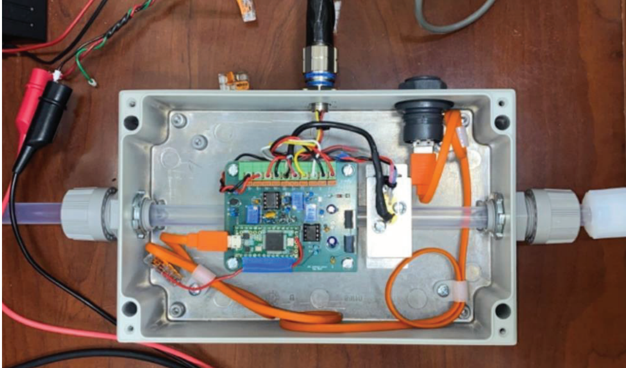
Figure 7.4-7. Second Assembled Pretreat Concentration Sensor
