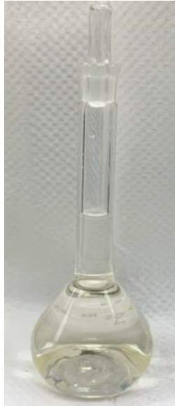
Figure 7.1-1. Container with 4 ppm of Iodine Dissolved in Pure Water
