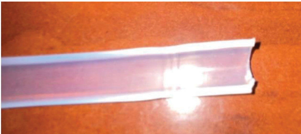
Figure 7.4-6. Damage Caused to PFA Tubing by Grommets
