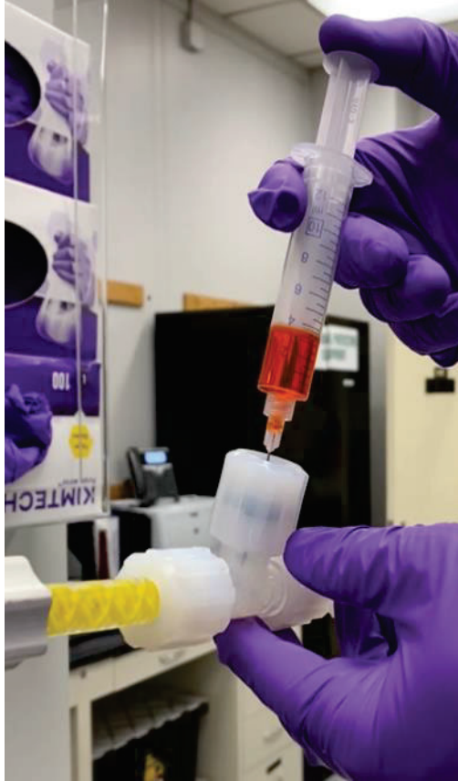
Figure 7.5-8. Manually Injecting Pretreat into Water Stream measured pretreat concentration
