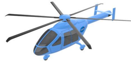
Quiet Single Main Rotor Helicopter
