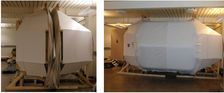
The Daedalus module in its stowed (left) and deployed (right) forms, which will be used as a teaching tool.
