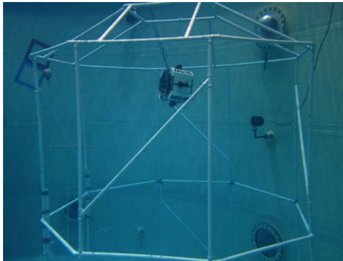
Figure 22. EUCLID vehicle performing controlled flight inside the underwater habitat mockup
