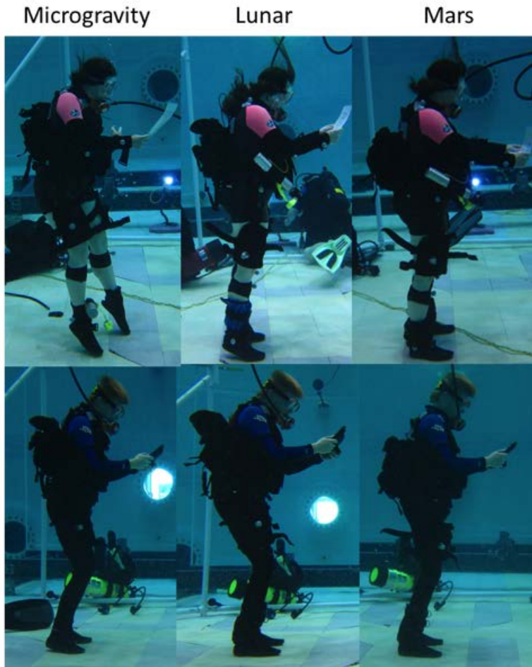
Figure 26. Neutral body posture in simulated microgravity (left), lunar (center), and Mars (right) gravity levels
