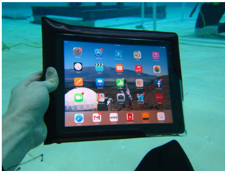
Figure 23. Tablet in waterproof housing during initial operational testing
