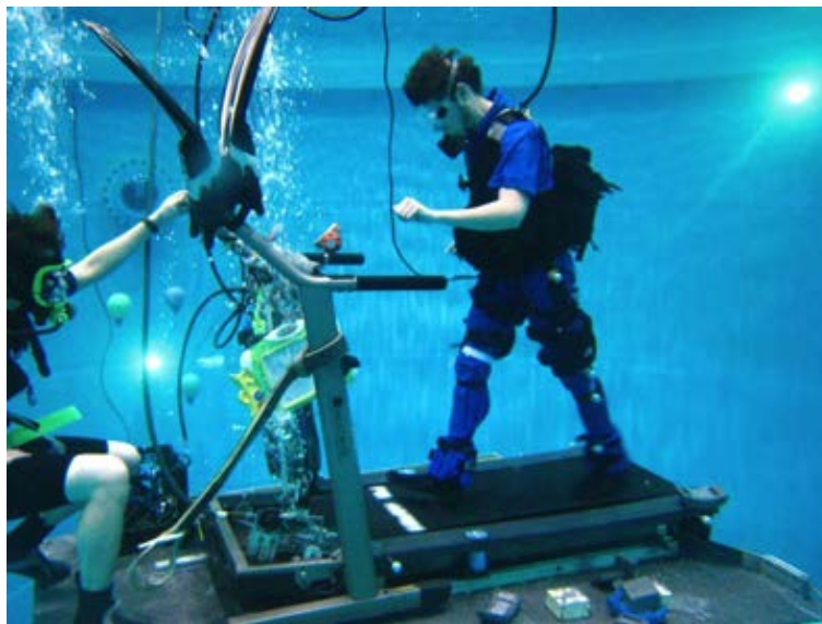
Figure 21. Underwater gait analysis of ballasted test subject at lunar gravity. Note lights from motion capture cameras used to illuminate tracking targets for position measurements.
