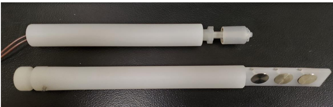
Figure 5. Fabricated Housing for the Float Switch Next to a Coupon Sample Rod
