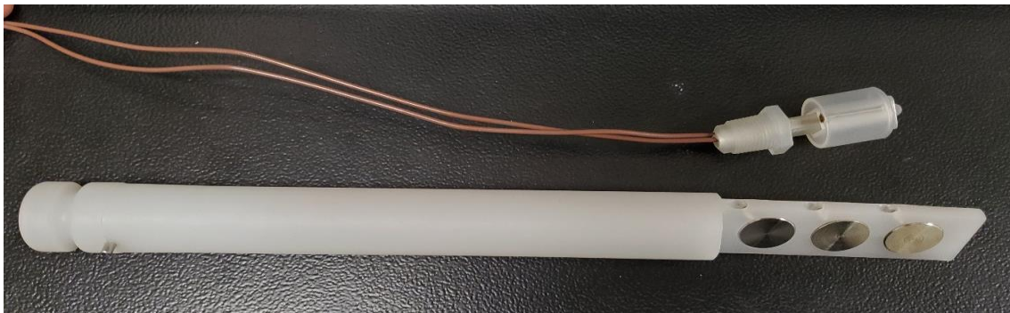
Figure 6. Prosense® Float Switch Next to a Coupon Sample Rod
